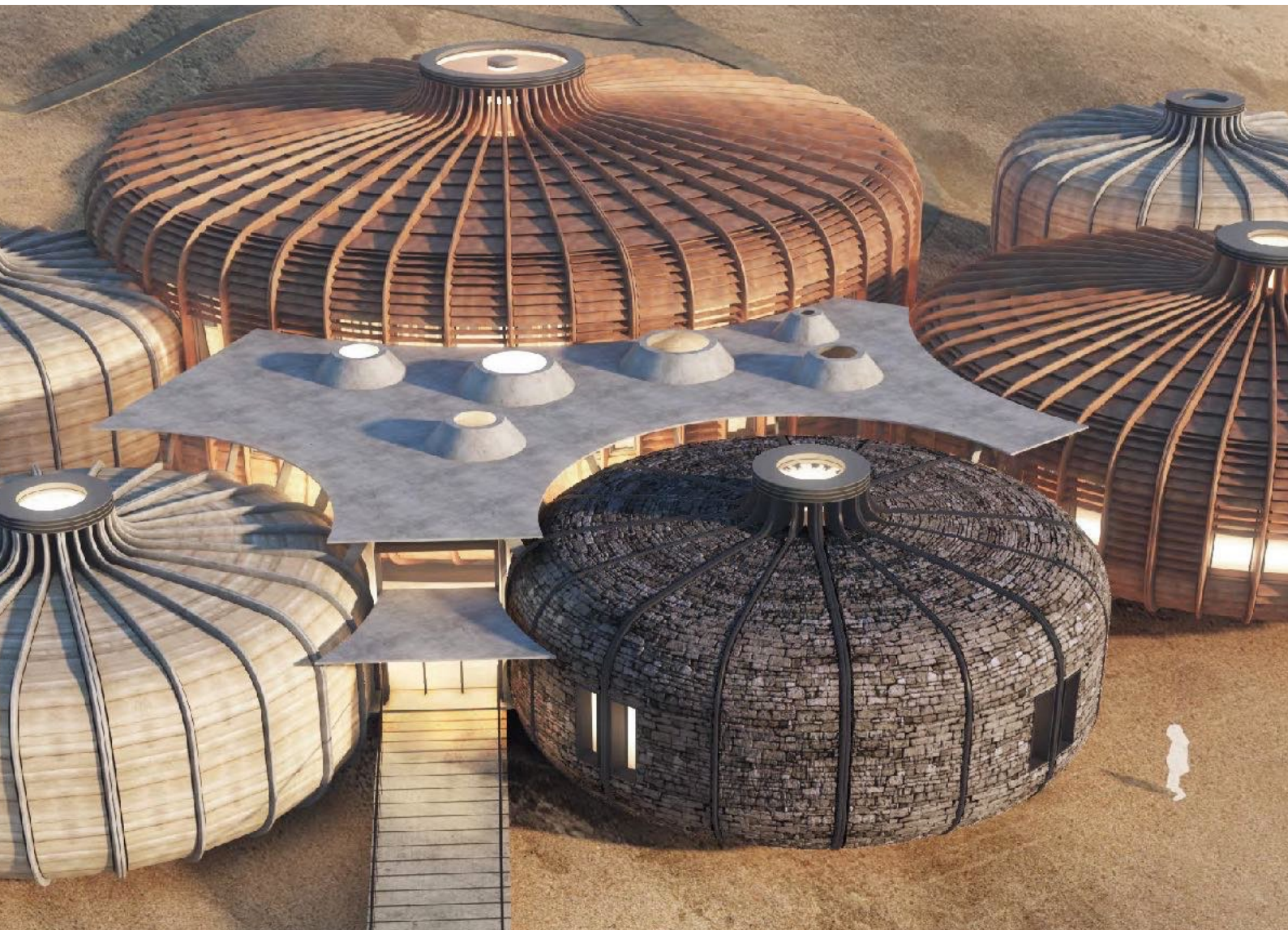
The idea is to provide daylight from the aperture of each module into the indoor spaces.
